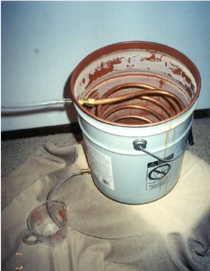
PHOTO: STEAM CONDENSER TO MEASURE ABSORBED HEAT
