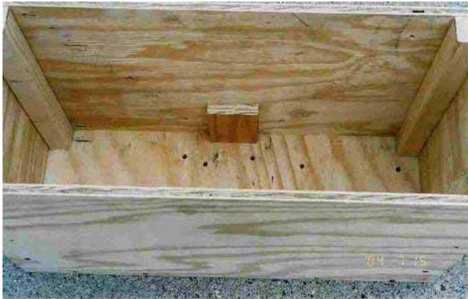
G. Attaching rear leg stop
