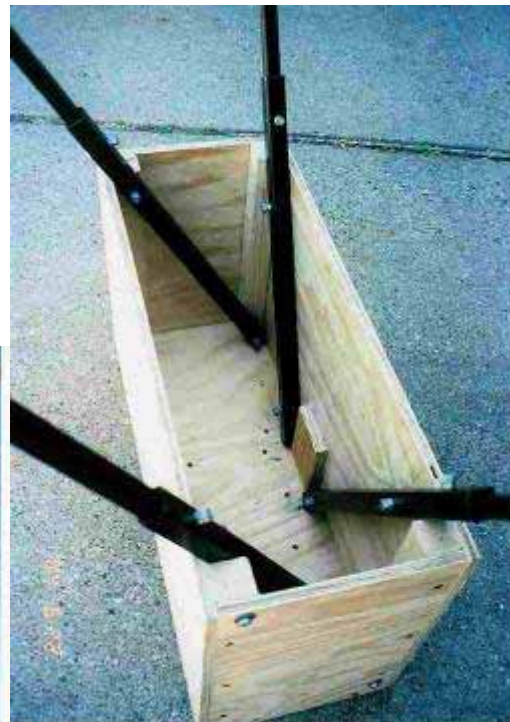
K. Attaching front upper legs
