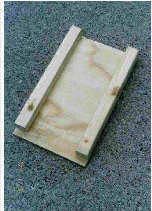
D. Attaching braces to end pieces
