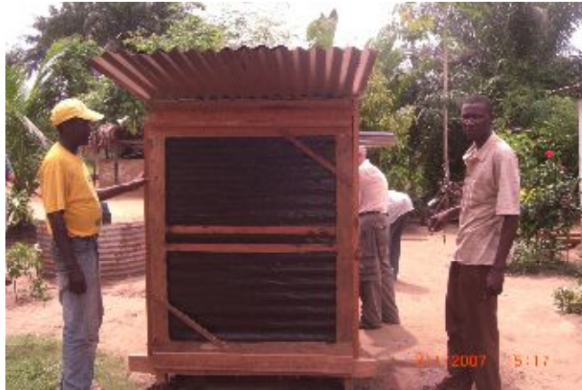
Barwain Zayzay (left) and Fallah Saah with front view of Solar dryer. Barwain is holding the door to the dryer. Fallah has gained expertise in the construction of the solar dryers
